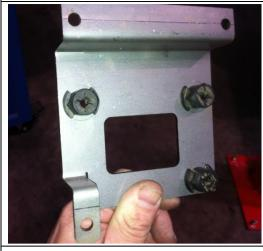
57. Fit the plastic lugs removed about to the radar sensor bracket as shown by inserting the lugs and turning ¼ turn clockwise.
