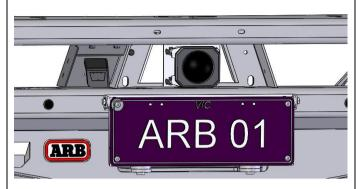
If fitting a winch and a radar sensor attach the folding license plate bracket supplied in kit 3540050 to the lower pan using M6 SS button head screws, M6 SS flat washers and M6 flange nuts.
