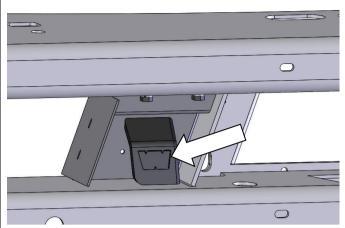
66. Attach the socket cover to the socket.
