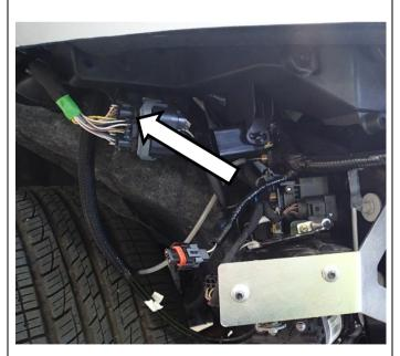
On each side of the vehicle, locate the wiring loom connectors.
