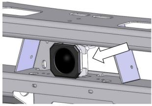
58. From the rear, carefully place the radar sensor into the bar as shown.
