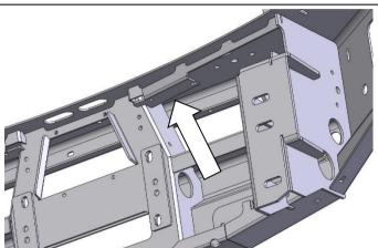
The control pack mounts to the bar here as shown using M6 hex bolts, M6 spring washers and M6 flat washers and M6 flange nuts.
