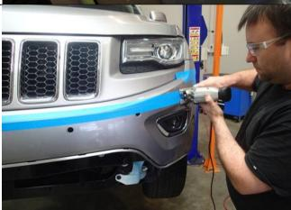
24. Using a jigsaw carefully cut along the lines marked above removing the lower section of the bumper.
