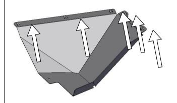
79. Add M6 cage nuts into the top surface of the RH and LH under wing panels as shown.
