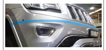
16. Using masking tape, mark a line following the horizontal feature line (corner) on the bumper bar following level to the ground to the wheel arch edge as shown.
