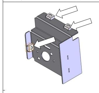
63. Fit M6 cage nuts to the plug mount bracket.
