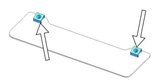
89. Place M6 cage nuts into each of the inner guard retention plates.
