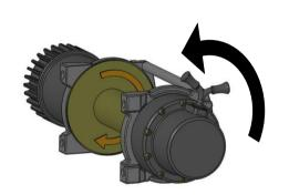
Warn / Magnum /Smittybilt winches: Undo the screws in the gearbox end of the winch. Carefully slide the gearbox away from the winch only until it is able to rotate. Rotate the gear box anti-clockwise 72° and replace screws.
