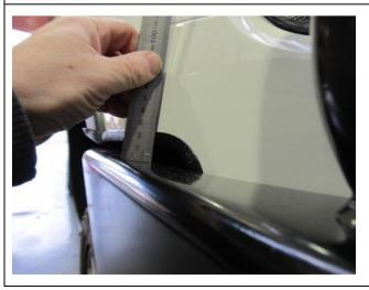
76. Adjust the bar so that it is central to the vehicle and has an even gap of between 8-14mm between the rear edge of the bar and the vehicles bumper.
