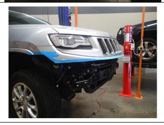
25. Using sandpaper or a file, remove any sharp edges.
