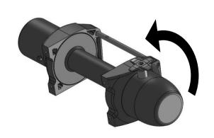
Bushranger winches: Undo the screws in the gearbox end of the winch. Carefully slide the gearbox away from the winch only until it is able to rotate. Rotate the gear box anti-clockwise 90° and replace screws.
