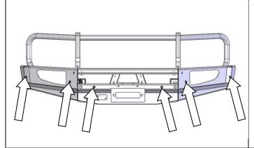
52. If not fitting parking sensors to the bar, fit the 6 plastic plugs to the bar into the parking sensor holes.
