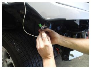
33. On each side of the vehicle identify the wire for the indicators and the clearance lamps using the chart below.
