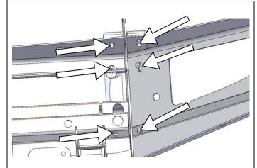
Attach the buffers to the bar using M6 flange nuts.
