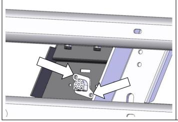
Attach the remote socket to the bracket using the screws removed from the factory control box. In the case of Zeon, use the M5 flange nuts supplied with the bar kit.
