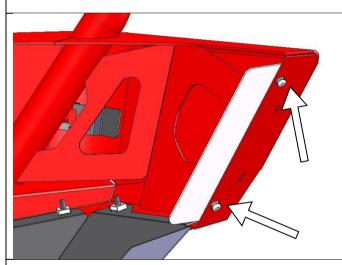
90. Attach the inner guard retention plates to the bulbar as shown using M6 button head screws, M6 spring washers and M6 flat washers.
