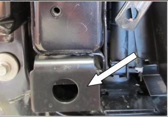
29. Remove any OEM tow points if fitted.
