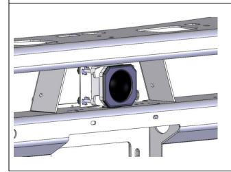
61. Carefully push the radar sensor into the plastic lugs ensuring that they all clip in firmly.
