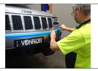
17. Run a second piece of tape parallel to the first piece leaving a 1-2mm gap as the cut line.
