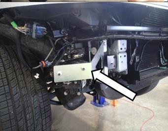
Attach the compressor bracket to the chassis and the compressor using the nuts removed earlier and the bolts removed in the step above.
