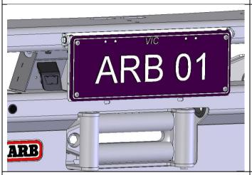
If fitting a winch only attach the folding license plate bracket supplied in kit 3540050 to the upper pan using M6 SS button head screws. M6 SS flat washers and M6 flange nuts.
