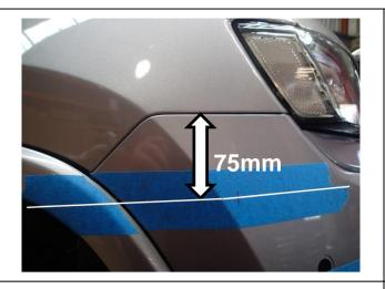
14. Using masking tape, mark a line 75mm down from the horizontal bumper joint line as shown. Run a second piece of tape parallel to the first piece leaving a 1-2mm gap as the cut line.
