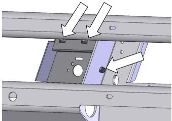
Attach the mount bracket to the bar using M6 hex bolts, M6 spring washers and M6 flat washers.
