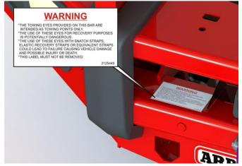
91. Place the tow warning label onto the top surface of the lower pan as shown.
