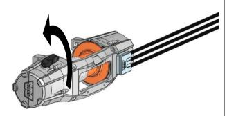
Warn Zeon winches: Undo the screws in the gearbox end of the winch. Carefully slide the gearbox away from the winch only until it is able to rotate. Rotate the gear box anti-clockwise 72° and replace screws.
